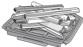
4. The hatch is set to the lighting position, that is the lower locking hook must be hooked securely around the lock reel. When the fire has caught fully after approx 10-15 minutes, close the doors completely (see figures to right). The first load of logs should not be put on until the start up fire has become a glowing bed of embers.
