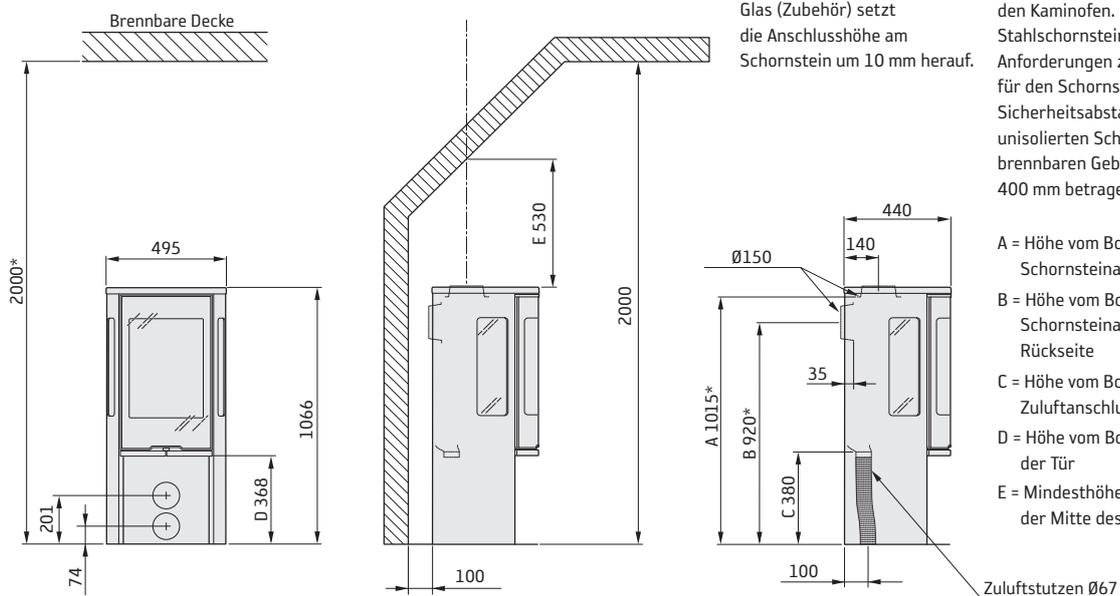
**INSTALLATION AN BRENNBAREN WÄNDEN**
