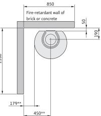
\* If the stove is placed on a hearth plate made of glass for example (accessory), the height from the floor is affected by a distance corresponding to the thickness of the hearth plate, for a free standing glass hearth plate this is 10 mm.
